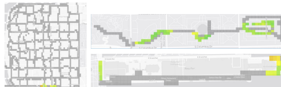
Figure 4. RSRP plot of T-Mobile n258 in the Loop (left), n258 in Grant Park (top), and n258 in Navy Pier (bottom)
